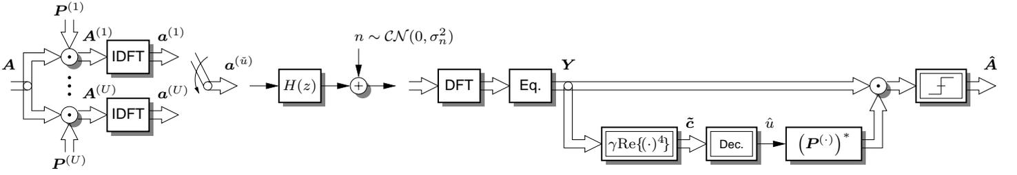
Fig. 1. Block diagram of candidate generation (left), transmission (middle), and decoding and inversion (right) of the side information.
