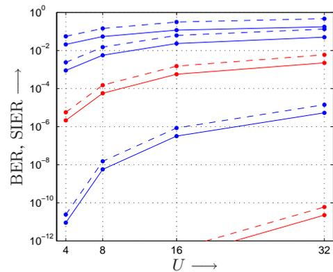
Fig. 6. Asymptotic SIER (dashed) or BER (solid) over the number  $U$  of assessed signal candidates for  $M = 16$  and (from top to bottom)  $D = 32, 64, 128, 256, 512$ . The subcarrier sizes analyzed in Fig. 5 are marked in red.
