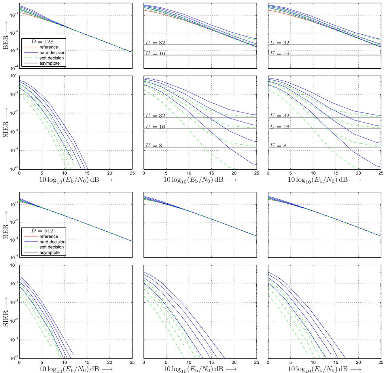
Fig. 5. BER (respective top rows) and SIER (respective bottom rows) over signal-to-noise ratio ( $E_b/N_0$ ) for SLM assessing  $U = 4, 8, 16, 32$  (curves from bottom to top) signal candidates; top plots:  $D = 128$ ; bottom plots:  $D = 512$ ; left column:  $M = 4$ ; middle column:  $M = 16$  with  $\delta = 0.5$ ; right column:  $M = 16$  with optimized  $\delta$  according to look-up table from Fig. 4.
