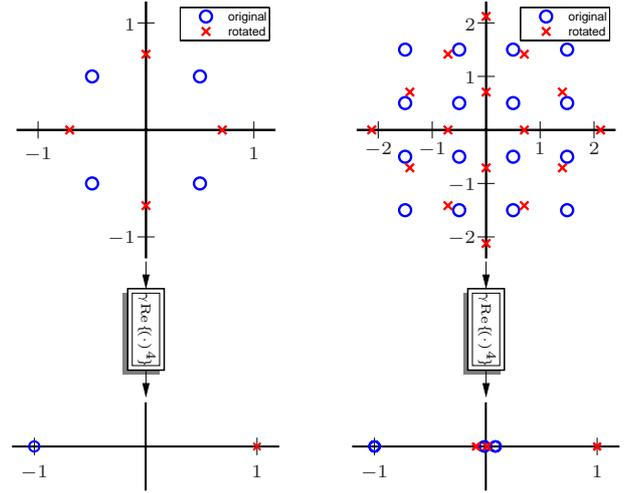
Fig. 3. Top: original QAM constellation ( $\circ$ ) and  $\pi/4$  rotated QAM constellation ( $\times$ ); bottom: resulting points after taking each point to the fourth power and dropping the imaginary part;  $M = 4$  (left),  $M = 16$  (right).
