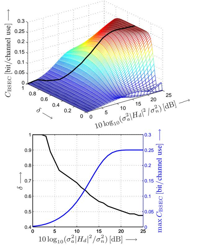
Fig. 4. Top: capacity of BSEC with bit error rate (8) and erasure rate (9) for various signal-to-noise ratios and borders  $\delta$  of the dead interval; the trajectory of maximum capacity is depicted black; bottom: resulting borders  $\delta$  (black) and maximum capacity (blue) over signal-to-noise ratio along the trajectory of the top plot;  $M = 16$ .
